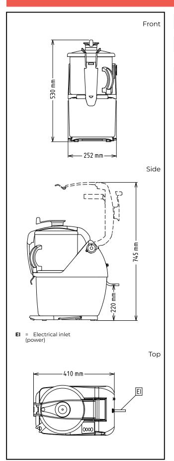
Electric Supply voltage: 200-240 V/1N ph/50/60 Hz Capacity: Performance (up to): 550 kg/hour 7 litres Capacity: Key Information: External dimensions, Width: 252 mm External dimensions, 485 mm Depth: External dimensions, 505 mm Height: **Shipping weight:** ISO 9001; ISO 14001 kg
